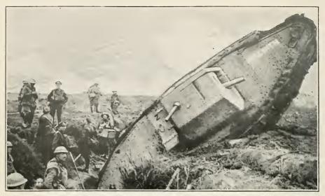
British tank unable to climb out of a German trench near Cambrai.
