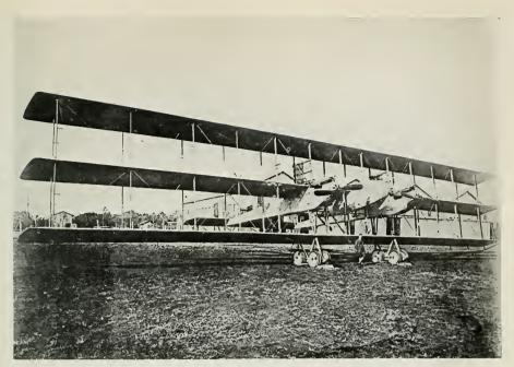
The Caproni triplane in America. Type of aeroplane used in bombing raids. Propelled by three motors with a total of 900 horse-power, capable of travelling eighty miles per hour, and carries three guns and about 2,700 pounds of explosives.
