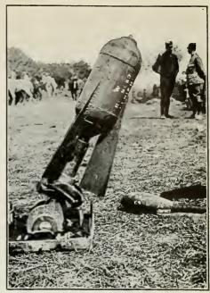
French trench mortar loaded with aërial torpedo.
